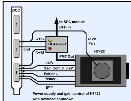
The output signal of the PMT is amplified by the HFAC-26-1 preamplifier. The single photon pulses at the output of the amplifier have a few 100 mV amplitude and are used to trigger the CFD input of a bh TCSPC module (SPC-300 through SPC-730, see manual at [www.beckerhickl.de](http://www.beckerhickl.de)).
