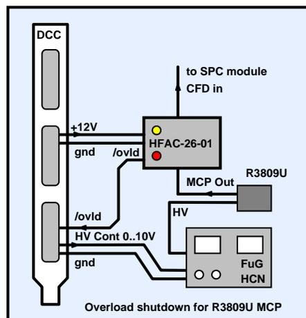
Don't connect or disconnect the signal cable from the detector to the preamplifier when the detector is switched on. This can destroy the amplifier. Make sure that you connected all ground connections. Missing ground connections can result in high voltage instability or unreliable overload shutdown.
