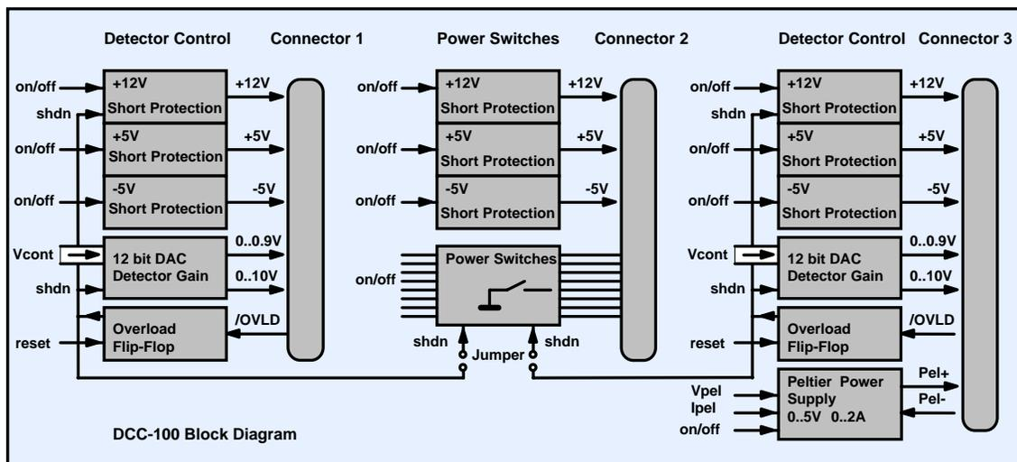
The DCC-100 contains two detector control blocks and one general purpose power switch block.
