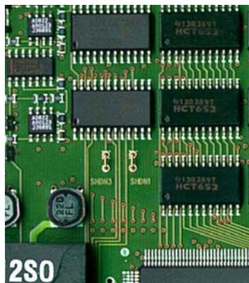
To operate the peltier cooling unit of an H7422 or PMC-100 detector the jumper next to the output connector must be removed (opened). Please make sure that the jumper at the connector which is NOT attached to an H7422 (PMC-100) is closed if only one detector is used. NEVER CLOSE BOTH JUMPERS SIMULTANEOUSLY.
