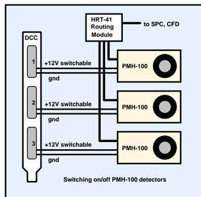
switching only one detector on, the desired detector can be selected for measurement. The configuration is exceptionally useful for laser scanning microscopes which normally use several detectors in different light paths.
