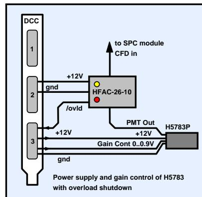
A second H5783 can be controlled separately via connector 1. In this case the power supply for both HFAC amplifiers should be taken from connector 2.
