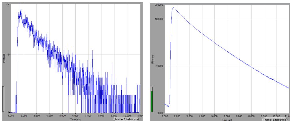
Fig. 6: Decay curves from the data shown in Fig. 5. Left: Decay data in a 10x10 pixel spot. Right: Decay curve from the entire image.
