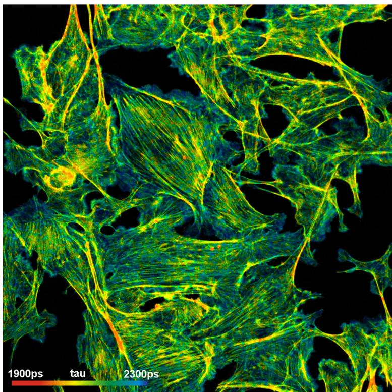
Fig. 5: FLIM of a BPEA sample, 1024x1024 pixels, 1024 time channels, acquisition time 10 seconds. DCS-120 system with BDL-SMN 488 nm ps diode laser and HPM-100-06 ultra-fast hybrid detector.
