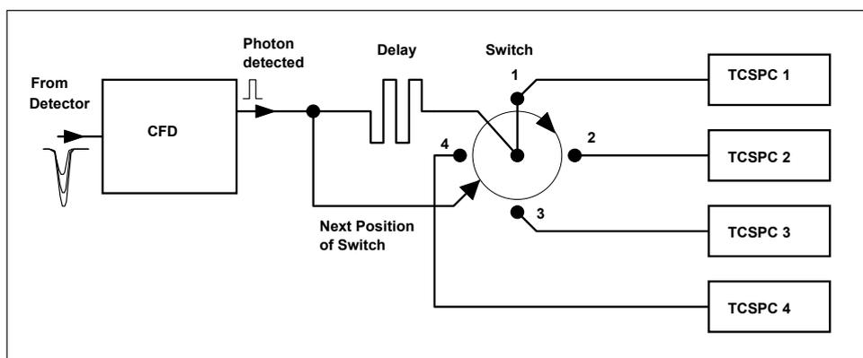
Fig. 1: The ‘Photon Spinner’. Every photon puts the position of a signal switch forward by one position. It arrives at the switch shortly after the switching action is complete, and proceeds into the next TCSPC module. Because the time between the switch set and the arrival at the switch is constant the switching transient has no effect on the photon timing.
