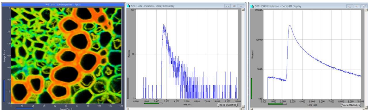
Fig. 2: FLIM of a Convallaria sample. Acquisition time 100 ms, 128x128 pixels, 1024 time channels, time channel width 12 ps. Lifetime range 1 ns (red) to 2.5 ns (blue). Middle and right: Decay curve in 5x5 pixel area and decay curve over entire image. DCS-120 system with 488 nm diode laser and HPM-100-40 detector.
