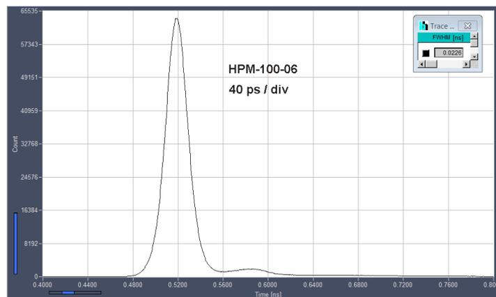
Fig. 8: Instrument response function of an SPC-154N four-module package with the Photon Spinner and an HPM-100-06 hybrid detector. FWHM is 22.6 ps.
