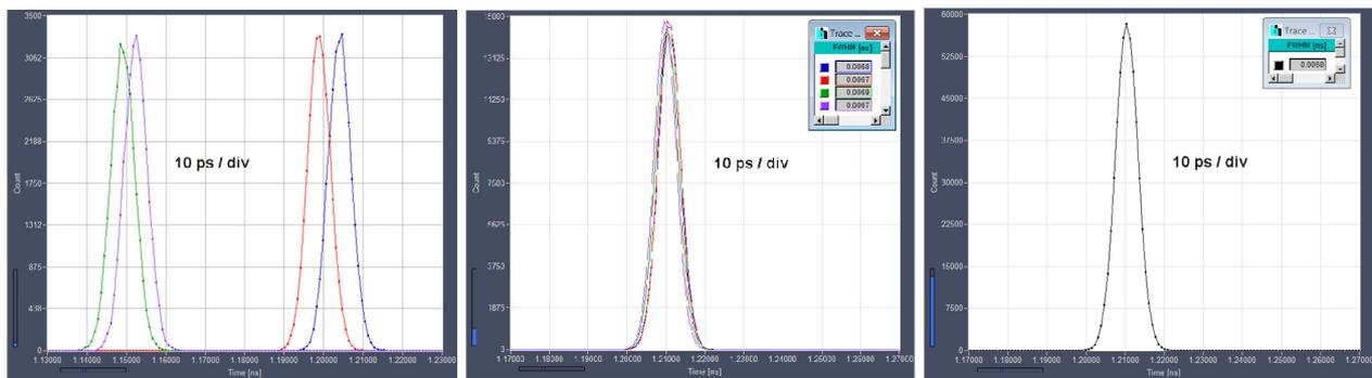
Fig. 7: Electrical IRFs of the four SPC-150N modules. Before (left) and after delay alignment (middle). The combined IRF of the four SPC-150N is shown on the right. The FWHM of the combined IRF is 6.8 ps.
