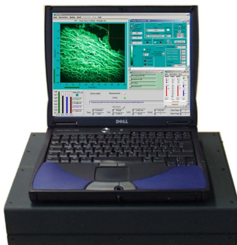
Fig. 6: Simple-Tau 150 system. The SPC-150 TCSPC-FLIM module and the DCC-100 detector controller are contained in a bus extension box of a lap-top computer
