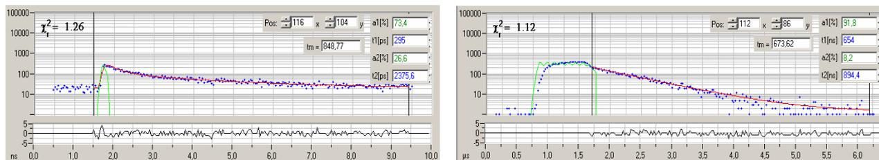
Fig. 10: Decay curves in selected spot of Fig. 9. Left: Fluorescence. Right: Phosphorescence. Blue dots photon numbers in the time channels, red curve fit with double-exponential decay model, green curve effective instrument response function. Inserts: Amplitude-weighted lifetime and double-exponential decay parameters. Decay parameters in ps for fluorescence and in ns for phosphorescence.
