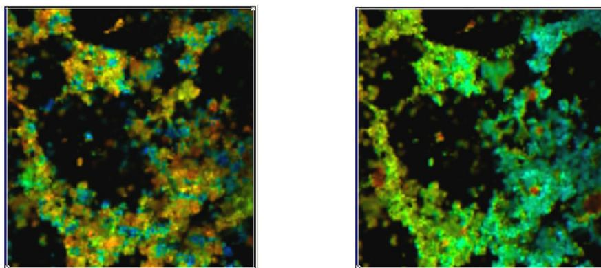
Fig. 7: Fluorescence lifetime image (left) and phosphorescence lifetime image (right) obtained from the data shown above. Colour scale red to blue 500 ps to 4 ns and 10 to 15 ms, respectively. SPCImage data analysis software.
