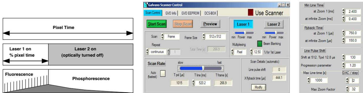
Fig. 4: DCS-120 system, scanner control parameters for phosphorescence decay imaging. Left: definition of laser modulation and scan rate control. Right: 'Scan Details', definition of maximum line time
