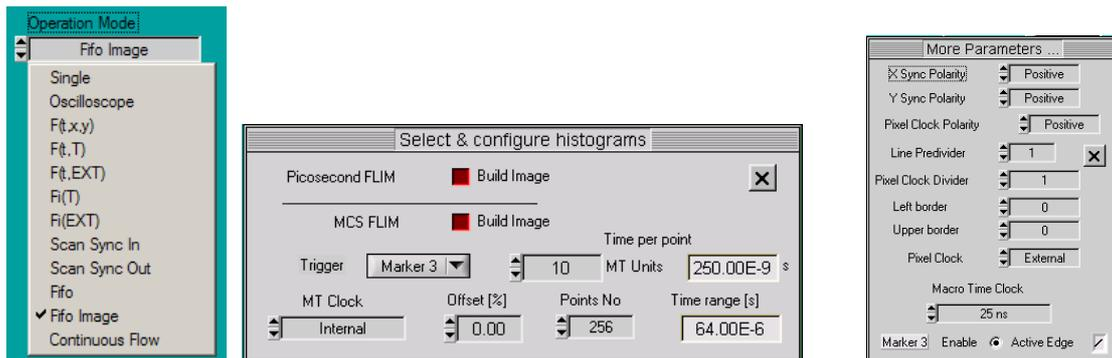
Fig. 3: Definition of MCS FLIM parameters. Left: Operation mode. Middle: Definition of timing parameters and marker selection. Right: Scan format parameters, macro time clock source, and marker enable.
