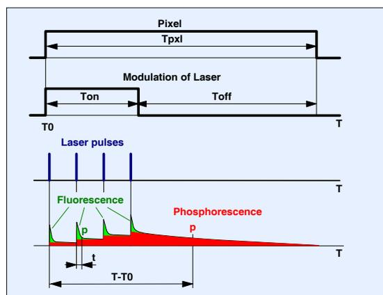
Fig. 1: Principle of Microsecond FLIM
