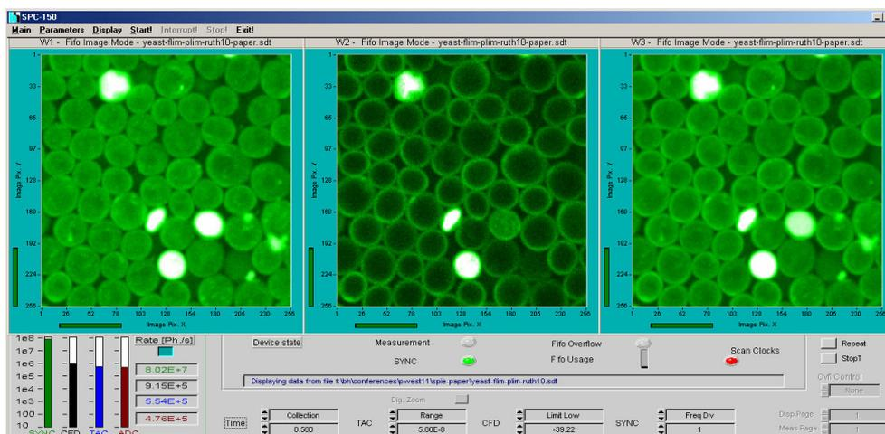
Fig. 8: Intensity images of yeast cells stained with a ruthenium dye. Images from left to right: Fluorescence, phosphorescence, total emission. LSM 710 NLO, two-photon excitation at 780 nm, non-descanned detection, HPM-100-40 hybrid detector, SPC-150 TCSPC FLIM module.
