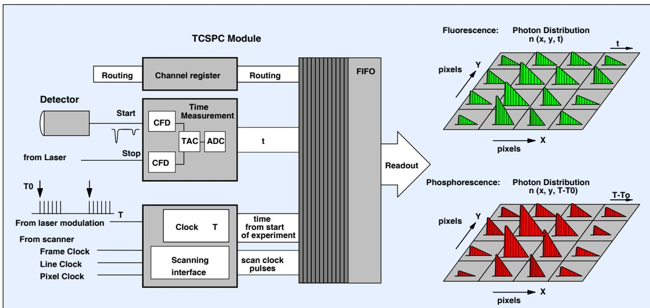
Fig. 2: Simultaneous fluorescence and phosphorescence lifetime imaging. Photon times are determined both with respect to the laser pulse period and with respect to the laser modulation period.
