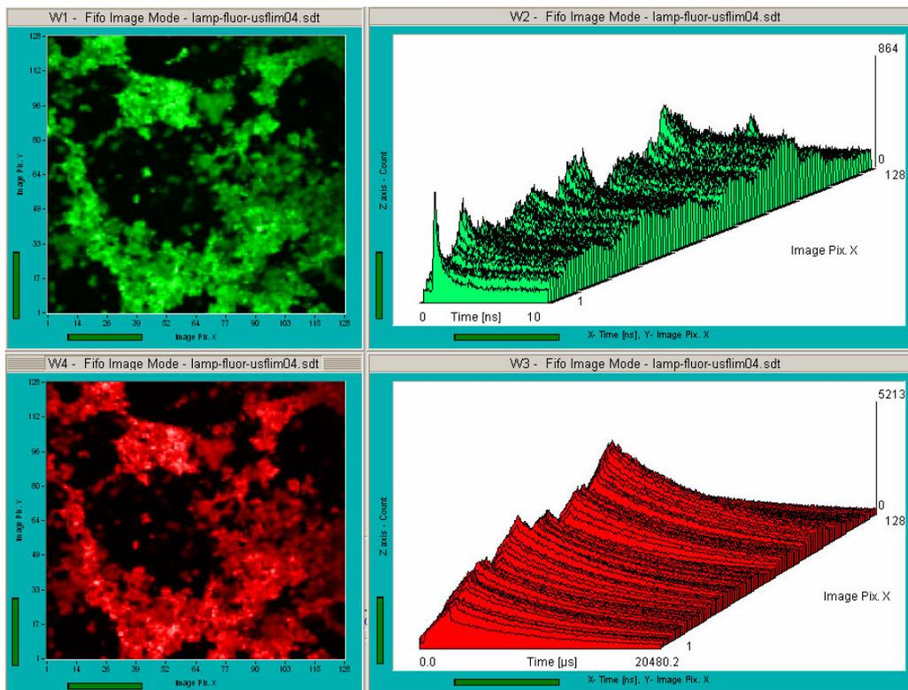
Fig. 6: Fluorescence image (upper left) and phosphorescence image (lower left) recorded simultaneously. ps decay curves and  $\mu$ s decay curves over a horizontal section of the image are shown upper right and a lower right, respectively. Particles of an inorganic luminophore, BDL-405SMC laser, Simple-Tau 152 FLIM system, SPCM data acquisition software.
