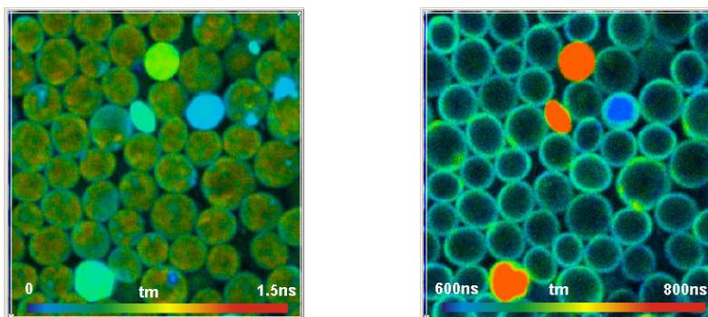
Fig. 9: Fluorescence lifetime image (left) and phosphorescence lifetime image (right) of yeast cells stained with tris(2,2'-bipyridyl)dichlororuthenium(II)hexahydrate. Amplitude-weighted mean lifetime of double exponential fit to decay data. Same data set as in Fig. 8, data analysis by Becker & Hickl SPCImage.
