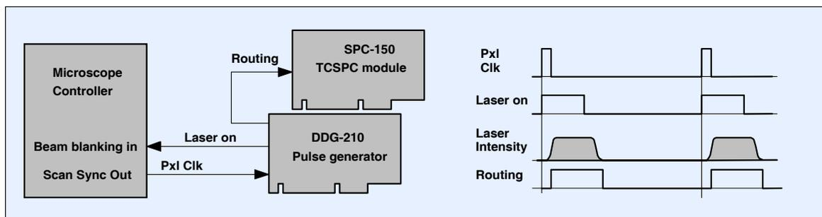
Fig. 5: On-off modulation of laser in other scanning systems than the DCS-120. The pixel clock of the microscope triggers the generation of a laser-on pulse in the DDG-210 pulse generator module. The laser-on pulse controls the beam blanking in the microscope. The AOM of the microscope responds to the beam blanking with a few  $\mu\text{s}$  delay. A routing signal to the SPC-150 TCSPC module indicates when the laser is on. Connection diagram shown left, pulse diagram right.
