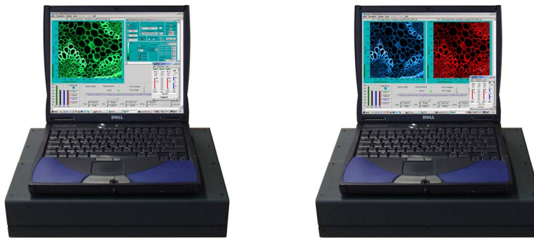
Fig. 7: Simple-Tau 150 and Simple-Tau 152 systems. One or two SPC-150 TCSPC-FLIM modules and a DCC-100 detector controller are contained in a bus extension box of a lap-top computer
