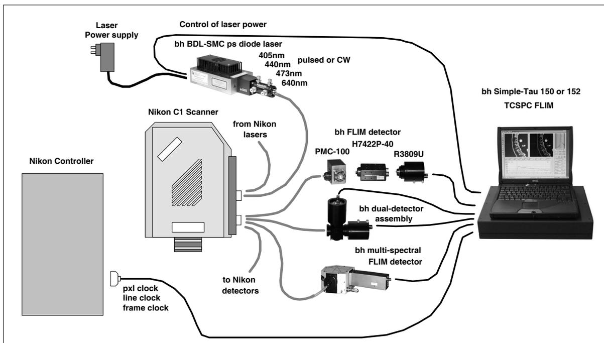
Fig. 1: Principle of the bh FLIM systems for the Nikon C1 scanners
