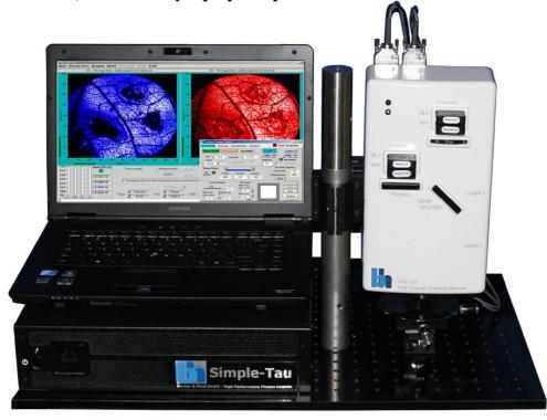
Scan field up to 15 mm diameter Pixel numbers from 16 x 16 to 2048 x 2048 Fast preview function Interactive scanner control Easy selection of scan field Beam-stop function for single-point measurement Single, double, or triple-exponential data analysis
