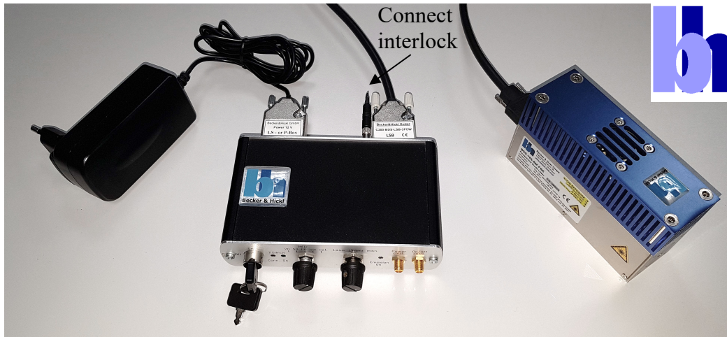
Fig. 3: BDS-SM laser. Left: Wall mounted power supply. Middle: Switch box with safety key, frequency switch for CW and pulsed operation, power control and SMA connectors for external control. Right: Laser module containing the complete driving and control electronics.
