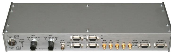
Fig. 3: Signal distribution and control box of the DCS-120 confocal scanning FLIM system
