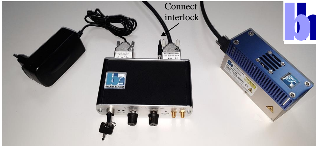
Fig. 1: BDS-SM laser. Left: Wall mounted power supply. Middle: Switch box with safety key, frequency switch for CW and pulsed operation, power control and SMA connectors for external control. Right: Laser module containing the complete driving and control electronics.
