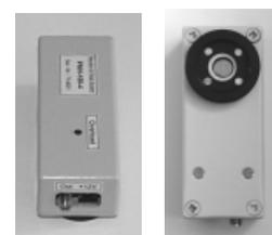
H5773, 150 to 240 ps FWHM. The PMH delivers single photon pulses in the range of -100 to -600 mV. If connected directly to the HRT, these pulses would drive the HRT amplifiers into saturation. Furthermore, the noise from the H5773 HV generator would trigger the HRT discriminators. Therefore, the PMH must be used with a 20 dB attenuator as shown in the figure right. With the attenuators directly in front of the HRT, the system benefits from the high noise immunity of the PMH-100 module.
