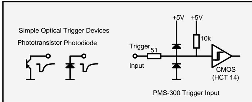
The input is protected by two safety diodes and a 50  $\Omega$  resistor. The 10 k $\Omega$  resistor pulls the open trigger input up to the 'high' level. Therefore, a simple photodiode or phototransistor can be used to derive a trigger signal from an optical pulse. The minimum trigger pulse width is 5 ns.
