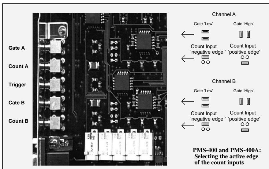
The input amplitude should be in the range between 20 mV and 1 V. Amplitudes above 1.5 V are clipped by safety diodes at the module input. Pulses up to 30 V (max. 1 us) and DC voltages up to 5 V will not damage the module. However, input amplitudes above 2.5 V should be avoided, since they can cause false counting due to reflections or crosstalk between the channels.
