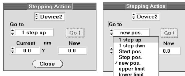
With 'Device 1' or 'Device 2' one of the two motors driven by the STP-240 can be selected. Several actions are available, as shown in the figure above (right). The action is initiated by the 'Go' button.
