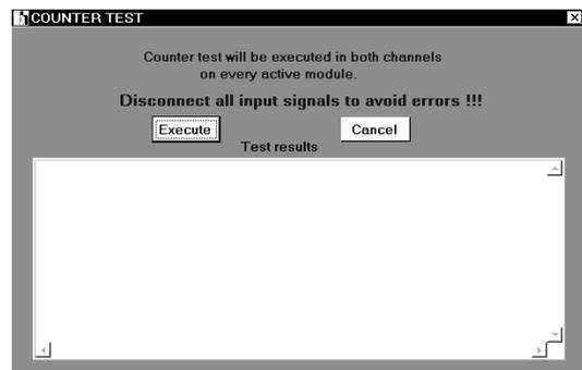
If the Counter Test does not return errors it is very unlikely that the module is damaged. The only parts that remains untested are the input protection resistors and diodes. However, these parts can be destroyed only by extreme overload, and it is unlikely that the overload protection is destroyed while the comparators are still working.
