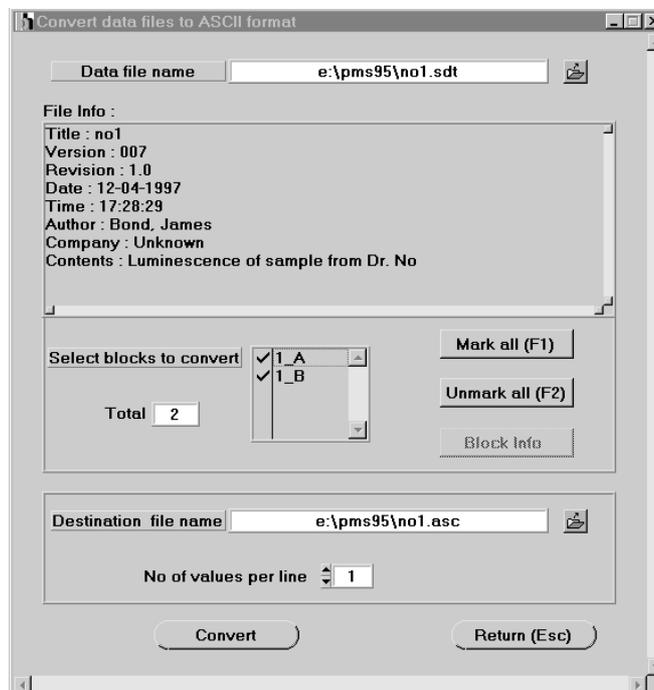
For 'Multiscaler' measurements the subsequent ASCII values resemble the subsequent counter values. For 'Event Mode' measurements pairs of values are generated which resemble the counter values and the times for the subsequent events.
