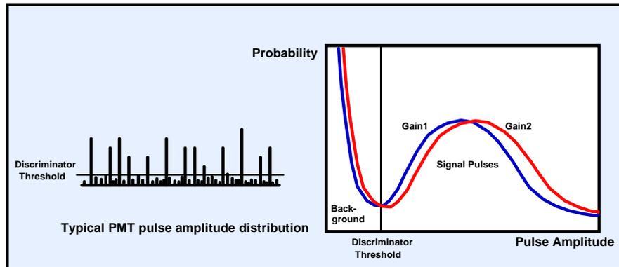
An additional source of noise are occasional detector pulses with extremely high amplitudes. These pulses are caused by cosmic ray particles, by radioactive decay or by tiny electrical discharges in the vicinity of the photocathode. Because these events are very rare they have no appreciable effect on Photon Counting. Analog Processing, however, is seriously affected by these high amplitude pulses.
