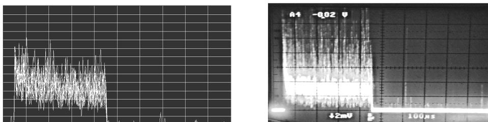
Recording of the same signal by a photon counter (left) and an oscilloscope (right).
