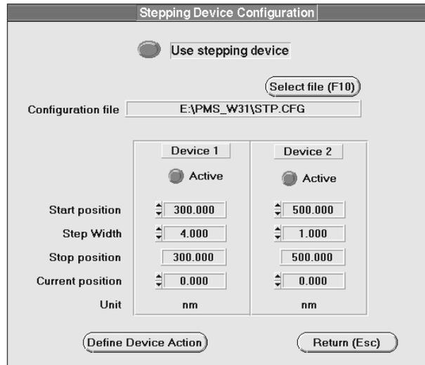
The basic electrical and mechanical parameters of the step motor drive are configured by a configuration file. This file contains the stepping frequency, start and stop ramps, duration of overvoltage pulses, end positions, the unit of the driven axis (e.g. nm for a wavelength drive) and the number of motor steps per unit. The default file name is STP.CFG. Other file names can be used to select between different configurations.
