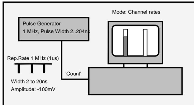
The pulses from the pulse generator are applied to one Count input of the PMS. The Gate input is left open. The PMS is operated in the 'Channel Rates' mode with
