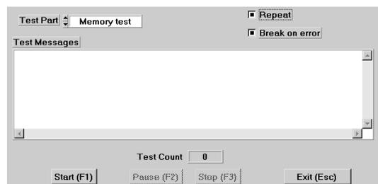
If an error should be displayed, check that the module is inserted correctly and that there is no address conflict (See next section).
