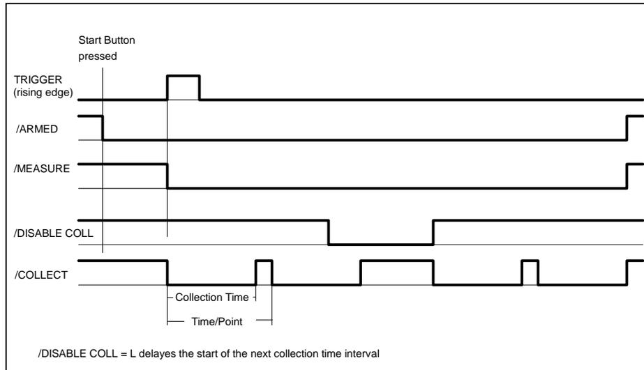
If /DisableColl is L at the start of a collection time interval the collection is not started. The measurement stops until /DisableColl = H is detected.
