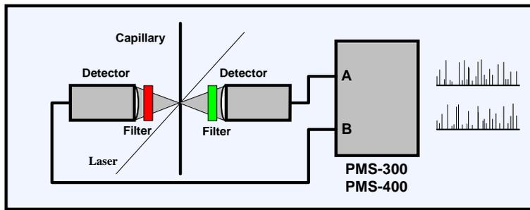
In all operation modes the gate inputs can be used to reject background pulses between the excitation pulses, to gate off straylight pulses during the excitation or to reduce fluorescence signals. Some examples are shown in the figure below.
