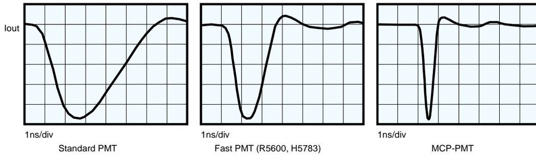
Fig. 3: Single Electron Response of Different PMTs
