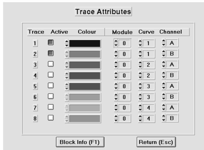
With 'active' a particular trace can be switched on or off. We recommend to switch off traces that are not needed. This will increase the speed of the display.
