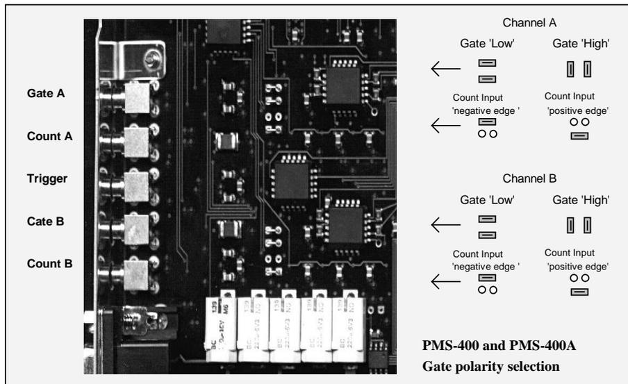
If the gate inputs are not used the gate must be set into the 'active' state by a gate threshold  $< 0$  in the active high configuration or by a gate threshold  $> 0$  in the active low configuration. If you do not know the setting of the jumpers on your module, run the 'Counter Test' function (under 'Main'), which returns the actual setting of the gate polarity jumpers.
