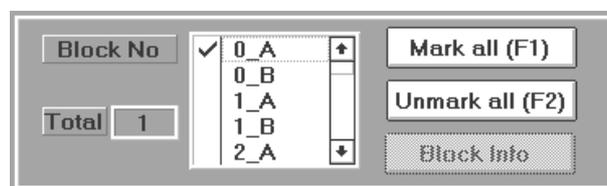
The list 'Block No' shows the curves which are available in the memory. The desired curves are selected (or deselected) from this list by a mouse click. 'Mark all' selects all curves, 'Unmark all' deselects all curves. 'Block info' displays information about a selected curve.
