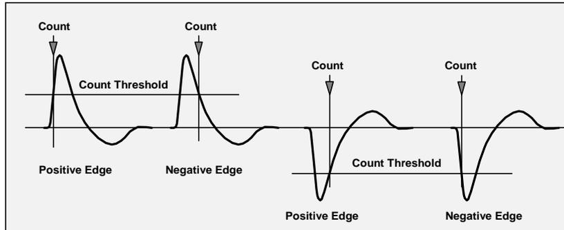
The active edge is selected by jumpers on the PMM board. The default setting is 'negative edge' as required for photomultipliers. The location of the jumpers on the board is shown in the figure below. Both channels can be set independently.
