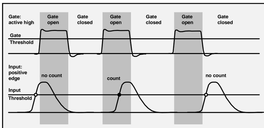
Because the gate of the PMS is edge controlled the gating resolution does not depend on the detector pulse width. The effective gate duration depends only on the gate pulse width, even if the gate pulse is shorter than the detector pulse.
