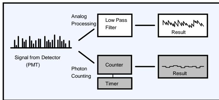
Analog acquisition of the PMT signal is done by smoothing the random pulse train from the PMT in a low pass filter. If the filter bandwidth is low enough the PMT signal is converted in a more or less continuous signal.
