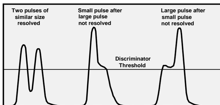
Effect of pulse height fluctuation on pulse resolution
