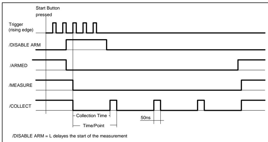
If /DisableArm is L when the 'Start Measurement' button is pressed the start of the measurement is delayed until /DisableArm is H. If a trigger condition is specified (the rising edge in the example above) the measurement starts with the next trigger after
