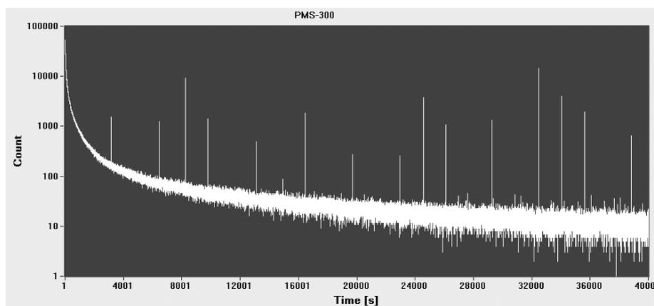
Decrease of dark count rate (counts per second) of a H5773P-01 after exposing the cathode to room light. The device was cooled to 5°C. The peaks are caused by scintillation effects.
