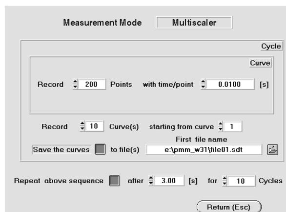
The 'Configure' menu is opened by clicking on the 'Configure' button in the main panel . The measurement sequence can (but need not) consist of three program loops:
