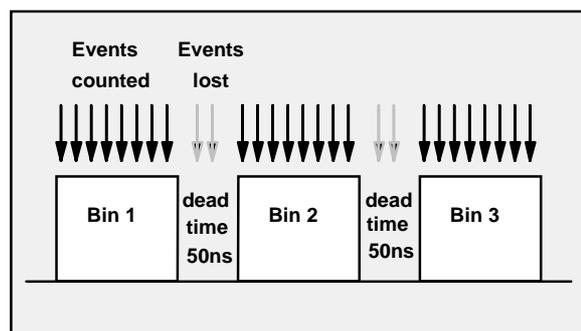
Counting loss due to dead time between subsequent bins
