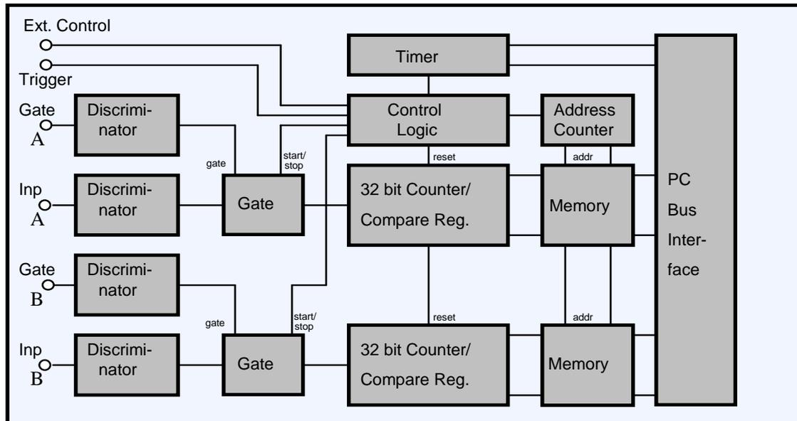
The counting inputs Inp A or Inp B receive the single photon pulses from the detectors. The input signals are fed to discriminators which respond when the input voltage exceeds a selected threshold. The input can be configured for positive or negative input pulses, the discriminator threshold can be set from -1V to +1V.
