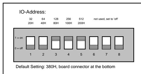
The software (standard software or library functions) reads the addresses of the used modules from the configuration file PMS300.INI. Therefore, the DIP switch setting and the addresses in PMS300.INI must be the same. The PMS300.INI file can be edited with any ASCII editor (e.g. Norton Commander).
