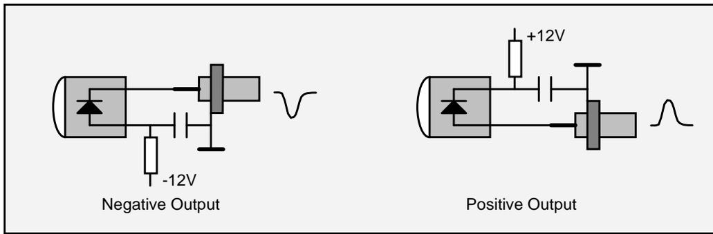
Complete photodiode modules are available from Becker & Hickl. These modules get their power from the PMS module so that no special power supply is required. For low repetition rates we recommend the PDM-400, for high repetition rates the PHD-400 which incorporates a current indicator for convenient adjusting. Please contact Becker & Hickl or see [www.becker-hickl.com](http://www.becker-hickl.com).
