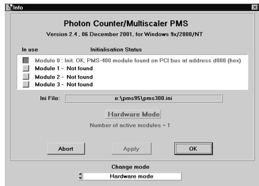
The software runs a simple hardware test when it initialises the modules. If an error is found, a message 'Hardware Errors Found' is given and the corresponding module is marked red. In case of non-fatal hardware errors you can start the main panel by selecting 'Hardware Mode' in the 'Change Mode' panel. Please note that this feature is intended for trouble shooting and repair rather than for normal use.
