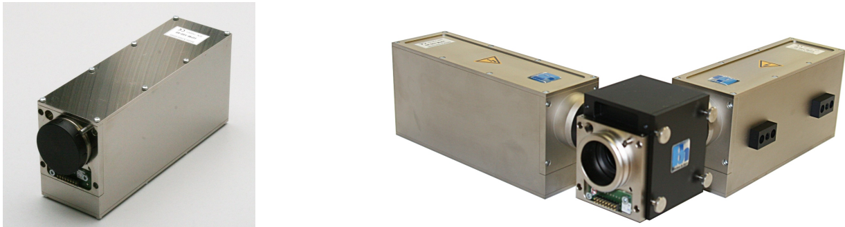
Fig. 5: Left: HPM-100 hybrid detector. Right: Two HPM-100 detectors coupled to a beamsplitter assembly.
