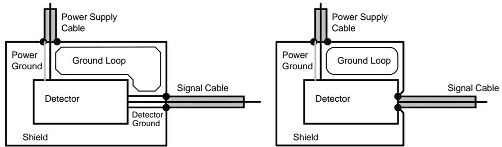
Fig. 7: Avoid that signal lines are part of a ground loop
