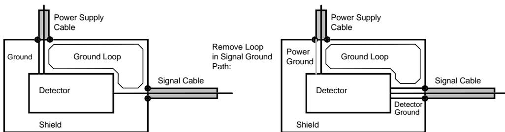
Fig. 6: Ground loop in the signal path
