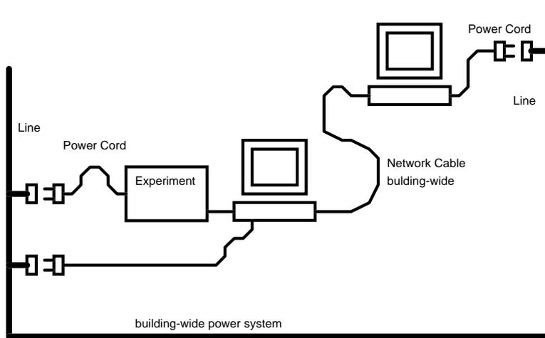
Fig. 5: Network cables often form building-wide ground loops
