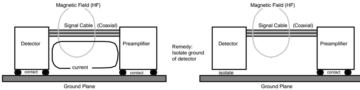
Fig. 1: Disrupting the ground loop by isolating the detector
