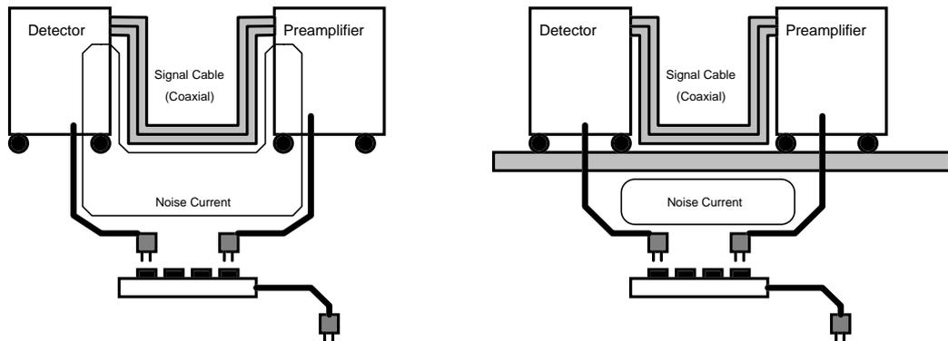
Fig. 4: Shorting power supply ground loop by the ground plane of the experiment
