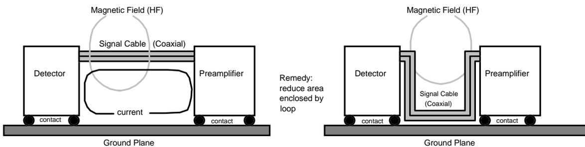
Fig. 2: If the ground loop cannot be avoided, minimise the enclosed area
