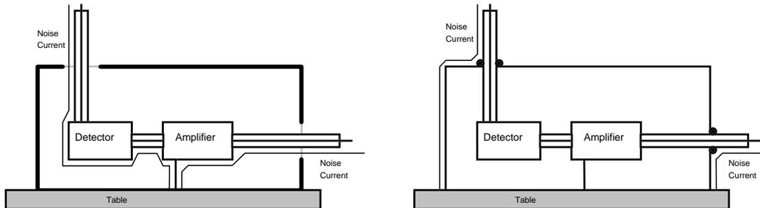
Fig. 8: Prevent ground loop currents from flowing into the shielding case
