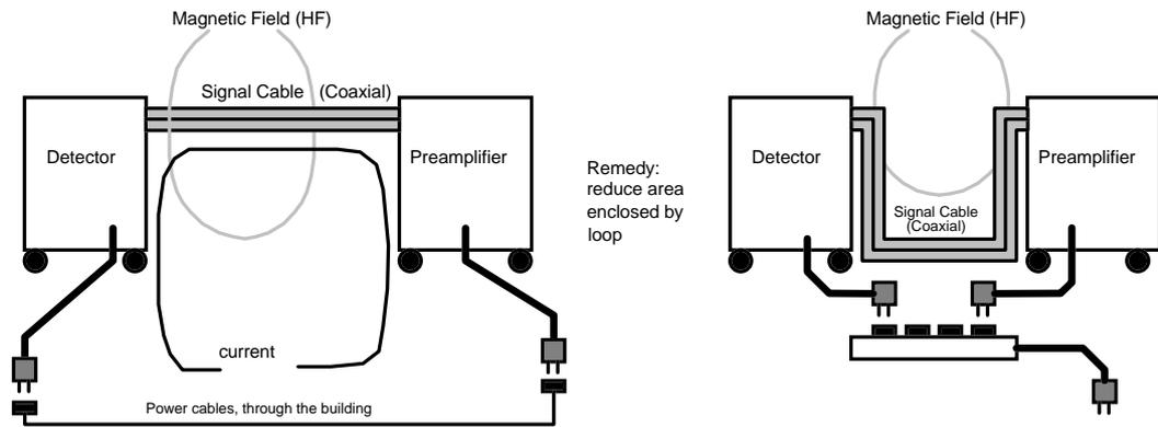
Fig. 3: Ground loop formed by power supply cables
