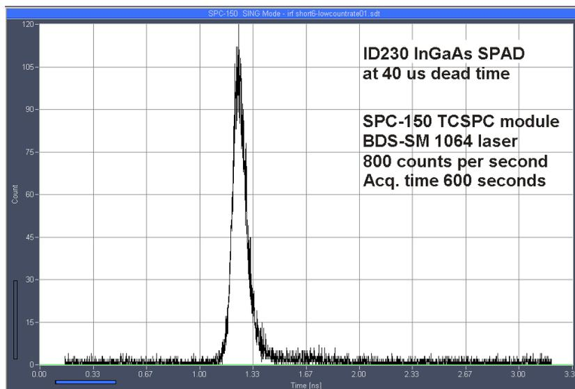
Fig. 4: Laser pulse recorded at a count rate of 800 photons per second. ID230 dead time 40  $\mu$ s, acquisition time 600 seconds. The long dead time decreases the counting background and thus results in a high signal-to-background ratio.
