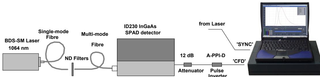
Fig. 2: TCSPC setup for characterising the id230 detector
