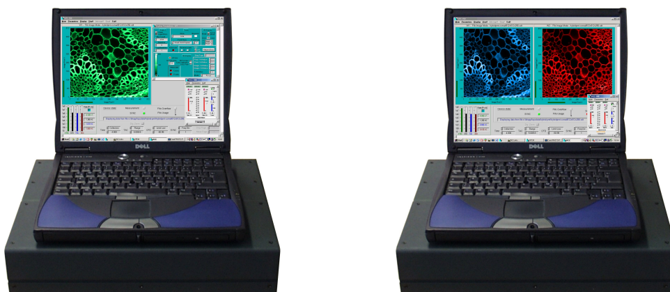
Fig. 2: bh Simple-Tau system. Single-channel system (left) and dual-channel system (right). The systems contain one SPC-830 or one or two SPC-150 TCSPC modules.
