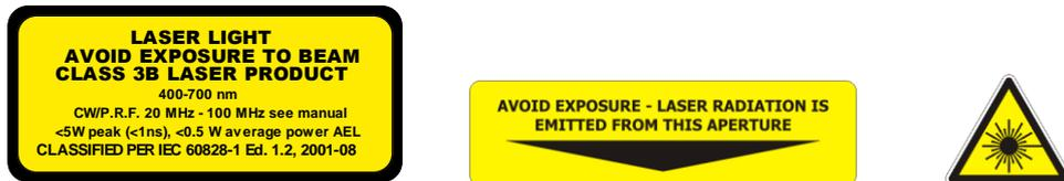
Fig. 40. Left to right: Explanatory label, aperture labels.
