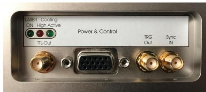
Fig. 5: Back panel of the BDL-SMN laser
