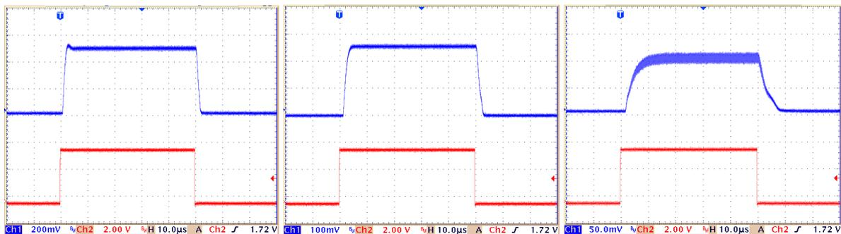
Fig. 7: Dynamic response of the output power to the power control signal. Control signal switches from 0 to +9V. Picosecond mode, 445 nm laser. Time scale 10µs per division. Red: Power control signal. Blue: Optical power. Left to right: Repetition rate 80 MHz, 50 MHz, 20 MHz. The noise in the 20 MHz curve is due to the pulsing of the laser.
