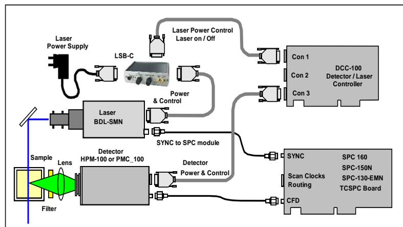
Fig. 28: Simple fluorescence-lifetime experiment
