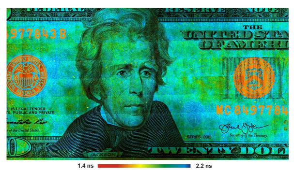
Fig. 45: Mosaic FLIM image of a \$20 bill. Combination of beam scanning with sample stepping by motor stage.
