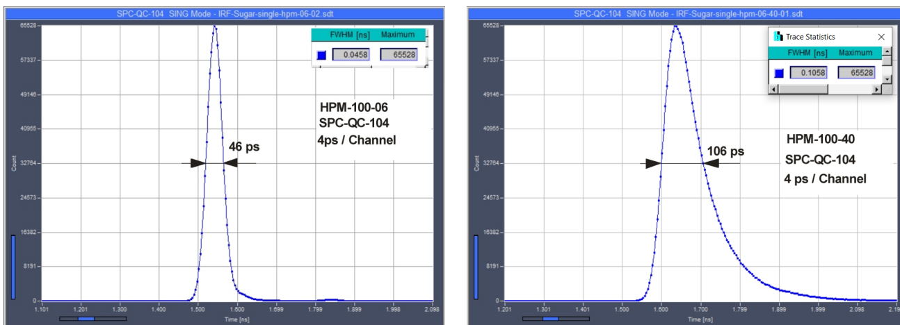
Fig. 127: IRF of HPM-100-06 (left) and HPM-100-40 (right) with SPC-QC-104. 100 ps/div, recorded at 379 nm.
