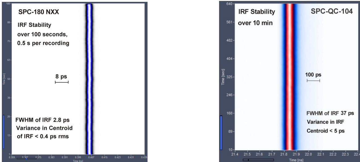
Fig. 31: Timing stability of an SPC-180NXX (left) and of an SPC-QC-104 (right). Time-series of measurements, display in Colour-Intensity mode. Note different time scale.
