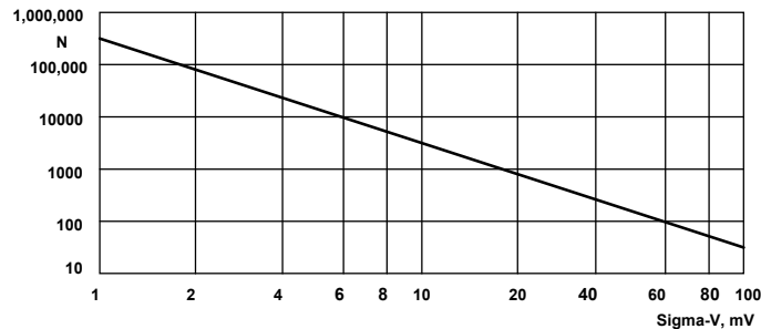
Fig. 4: Number of photons per pixel, N , needed for a desired standard deviation, \sigma_V , of the membrane voltage, V_m
