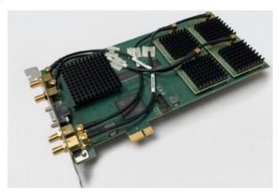
You should have a Becker&Hickl SPC-QC-104 inserted in a PClexpress slot of Windows 64-Bit computer running at least Windows 10 or later.
