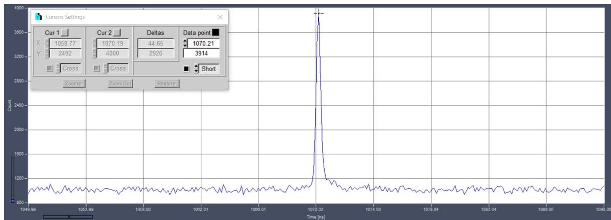
Fig. 4: Zoom into the region around the primary-target peak. The peak time is 1070.21 ns, corresponding to a target distance of 160.53 m.
