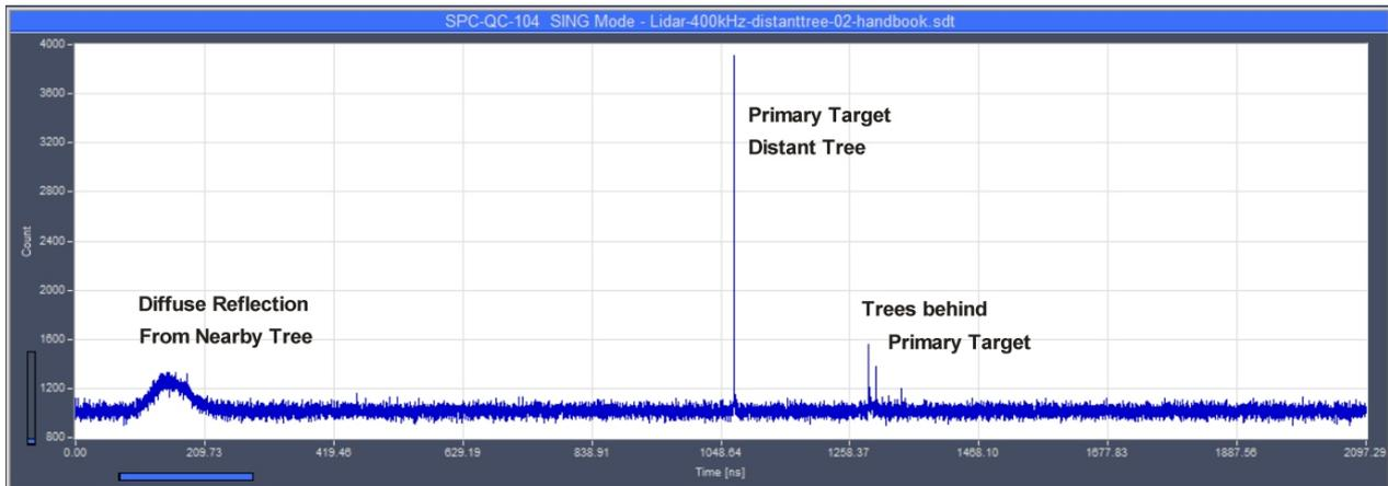
Fig. 3: LIDAR result obtained with the setup shown in Fig. 2. Laser repetition rate 250 kHz, laser pulse energy 40 pJ.
