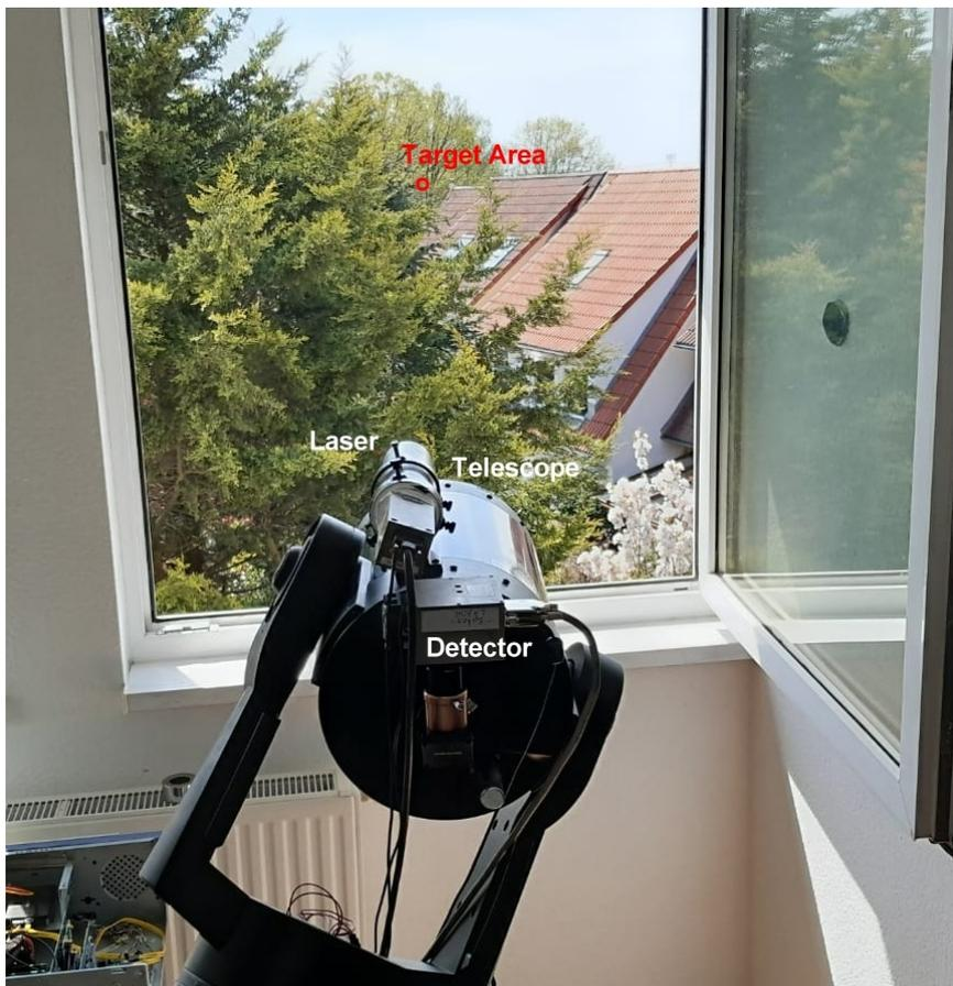
Fig. 2: Optical setup
