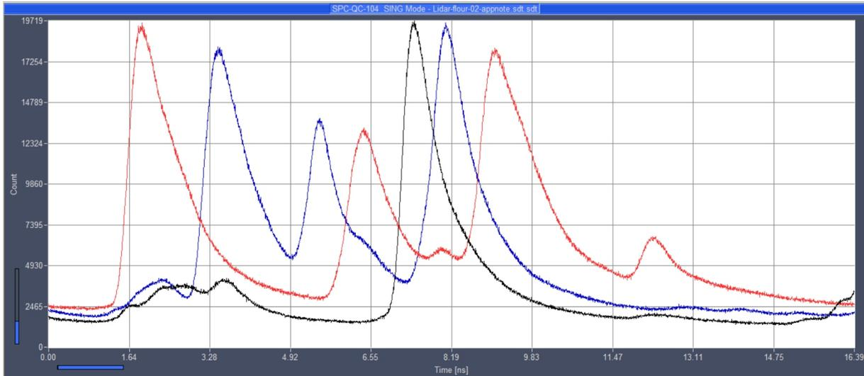
Fig. 5: Fluorescence decay curves of chlorophyll recorded from a tree 160 m away. The three curves were recorded from slightly different locations. The laser beam illuminated several leaves simultaneously, therefore several decay profiles are present in each curve.
