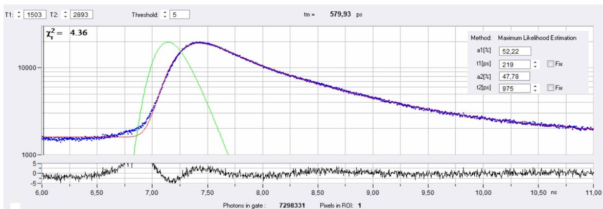
Fig. 6: De-convolution of the decay in the middle of the black curve in Fig. 5. Double-exponential model, synthetic IRF. Decay components shown in the insert upper right. The green curve is the IRF.
