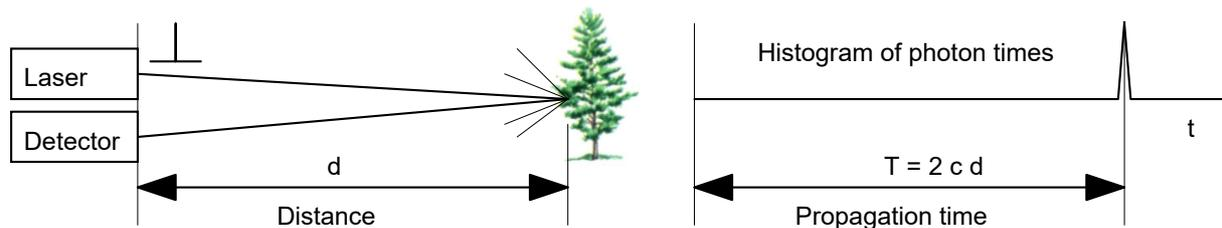
Fig. 1: Principle of LIDAR
